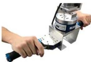
Fig.2 Handle attached to tip of manipulator
