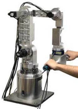
Fig.1 The manipulator for a hand guide system
